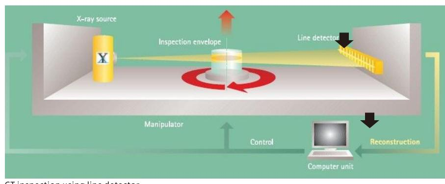
CT inspection using line detector
