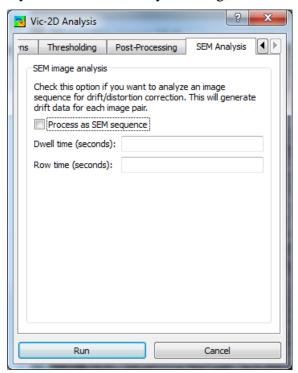
Check the **Process as SEM sequence** box. Enter the dwell time and row time, in seconds:
